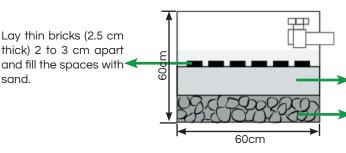
Intermediate layer with sand with an effective size between 0.3 and 1.6 mm (1/64" and 1/16") of 0.15 m thickness.
